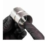
3.) Prepare barrel nut for installation using a small amount of grease (Aeroshell 64)
