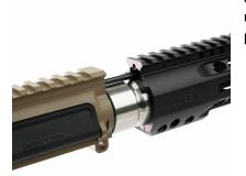
8.) Install the handguard over the barrel and barrel but. Align the upper rail to the handguard. Ensure the anti-rotation pin is in place.
